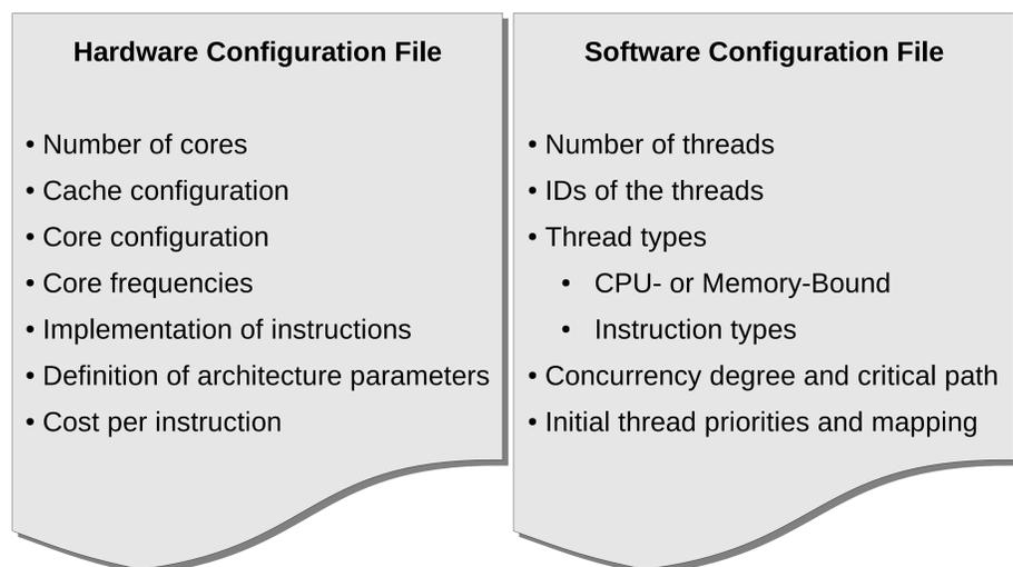
Figure 2: Hardware and software configuration files generated at compilation time. The software configuration file can be updated by the OS during the program execution whenever changes are detected by hardware/software monitors.
